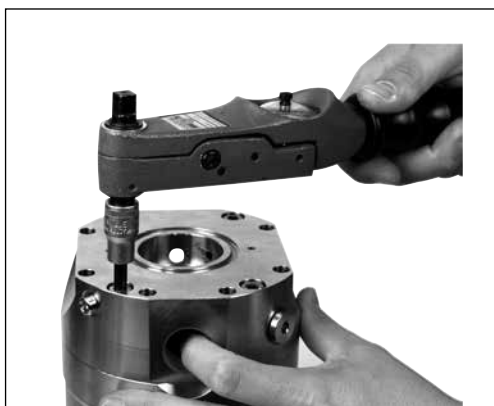
7. Tighten screws to 30Nm.
