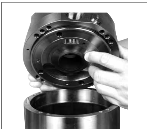
5. Mount port flange on housing. Use pin as guide.
